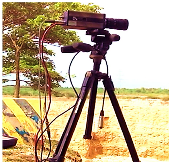
Figure 2. High speed video camera of 1000fps capacity
